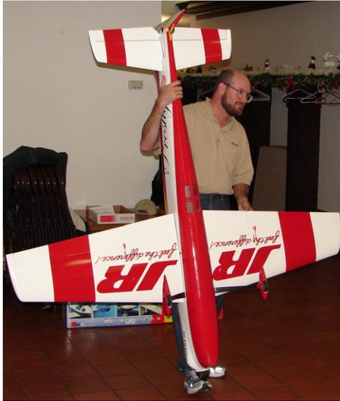
Full composite molded fiberglass/balsa
