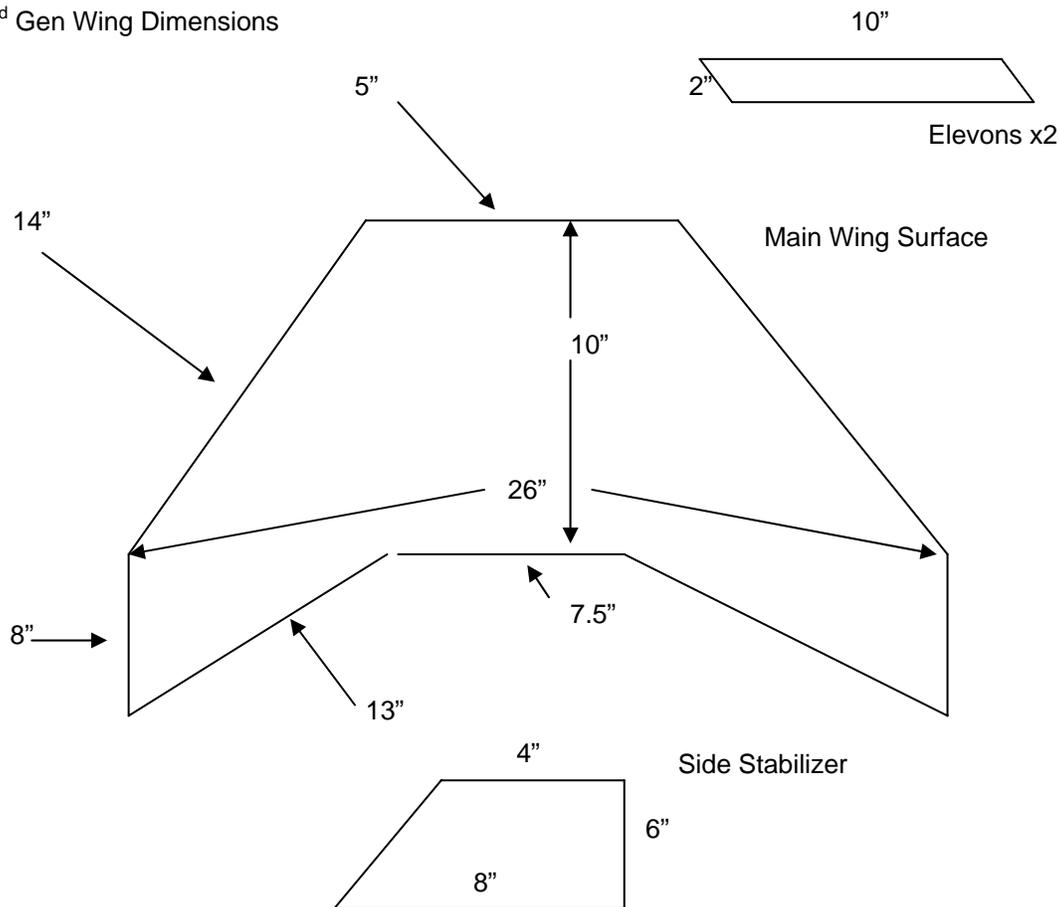
flex/crash resistance. The weight of the all-up wing is about 13-15 ounces. Nothing is really critical with the dimensions. I've built 4 versions of this design with slight shape differences and very little changes in flight performance. No airfoil here – just pure thrust. I have attached the rough dimensions if you decide you want to build a copy. You can use Depron lunch trays if you don't mind the smell of a hoagie when you fly your wing!
